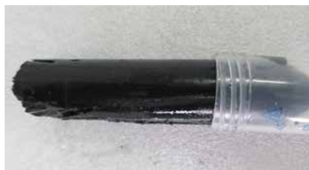
Figure 2. Tissue Samples Made from a Mixture of Agar and Graphite
